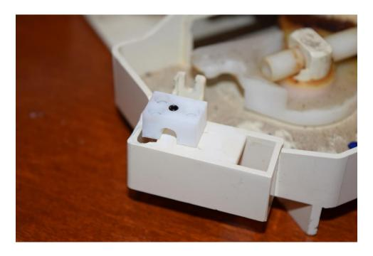
5.) Insert the appropriate lower clamp (**short**: air direction knob, **long**: heat/cool knob) into the opening directly below the upper clamp, with the double holes aligning with the double holes on the upper clamp:
